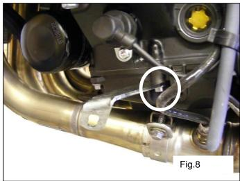
7. Allign belly pan to brackets and fit using M6 x 20 socket flange screw (12) and M6 nuts (13) to secure the belly pan to the brackets.
